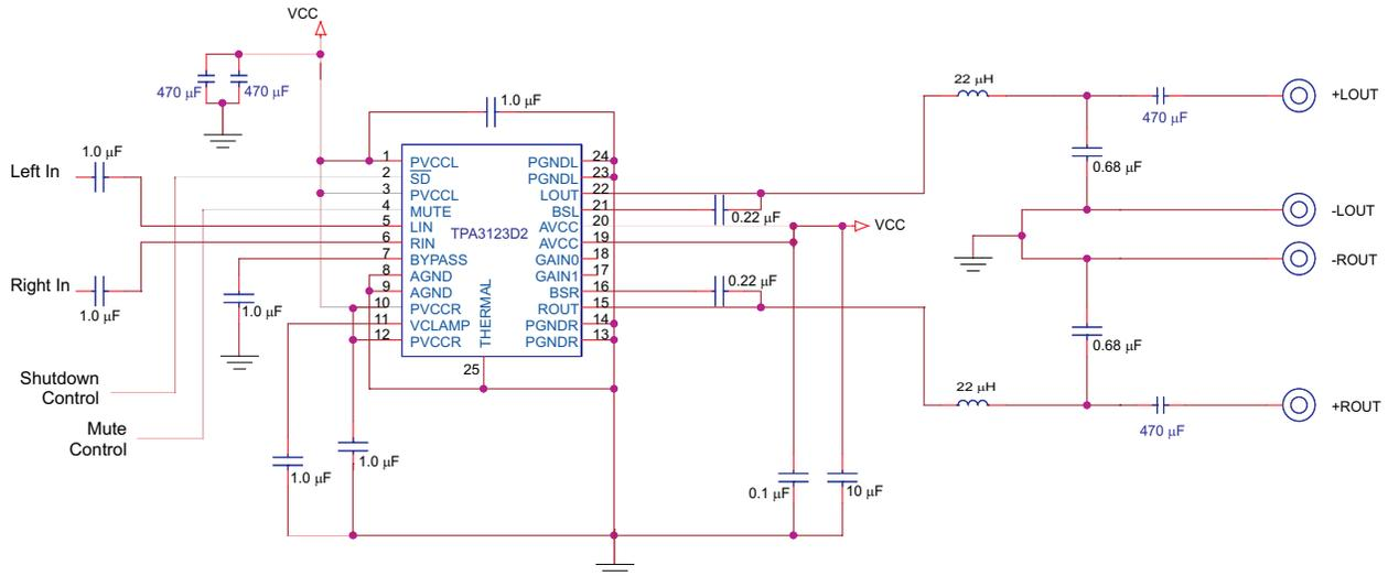
Figure 27. Schematic for Single Ended (SE) Configuration
