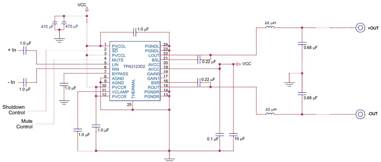
Figure 28. Schematic for Bridge Tied (BTL) Configuration
