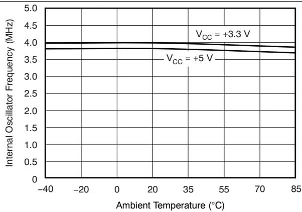
**Figure 10. Internal Oscillator Frequency vs Ambient Temperature**
