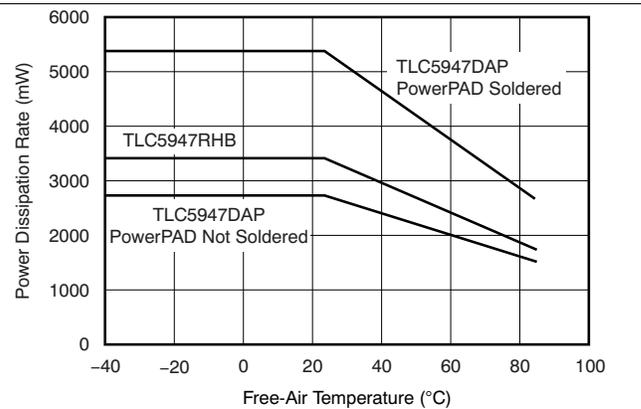
Figure 5. Power Dissipation Rate vs Free-Air Temperature
