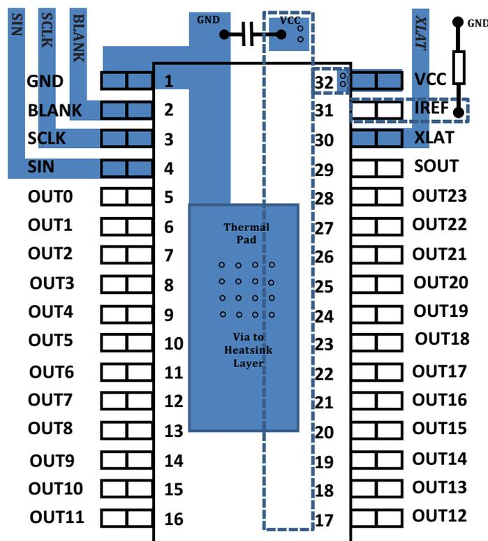
Figure 26. Layout Schematic
