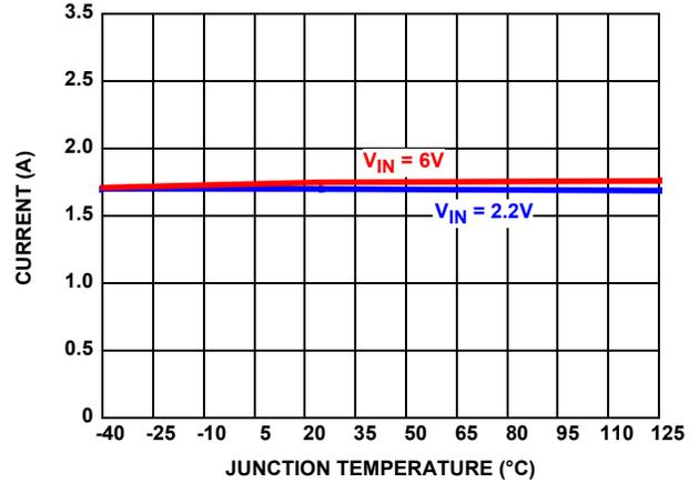
FIGURE 10. CURRENT LIMIT vs TEMPERATURE ( $V_{OUT} = 0V$ )
