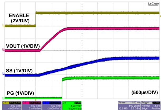
FIGURE 11. ENABLE START-UP ( $C_{SS} = 2.2nF$ )
