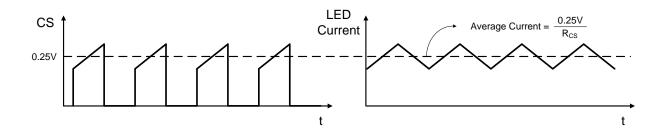
The above equations are only valid for continuous conduction of the output inductor. It is a good practice to design the inductor such that the switching ripple current in it is 25% of its average peak-to-peak, full load, DC current.
