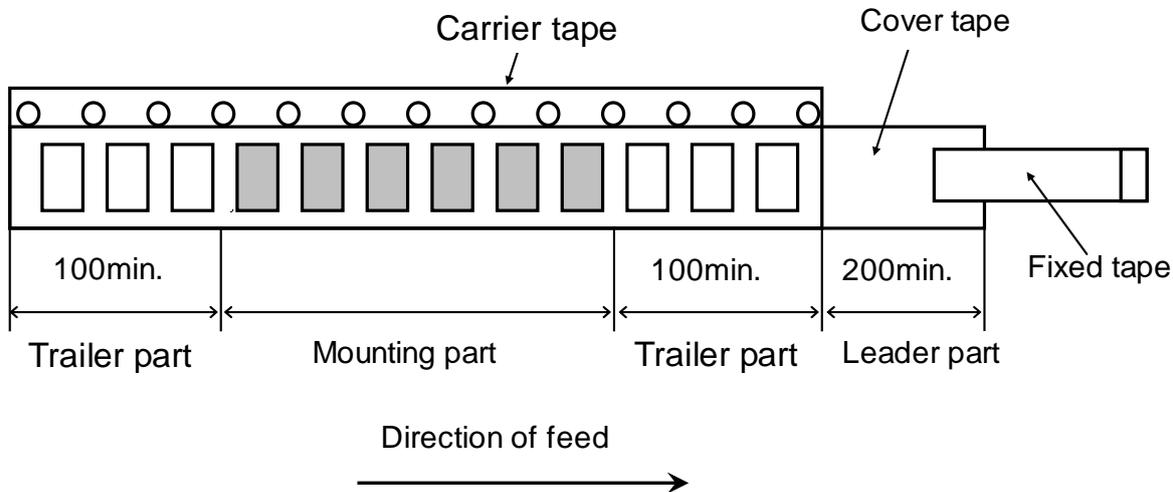
The cover tape shall not cover the sprocket holes
