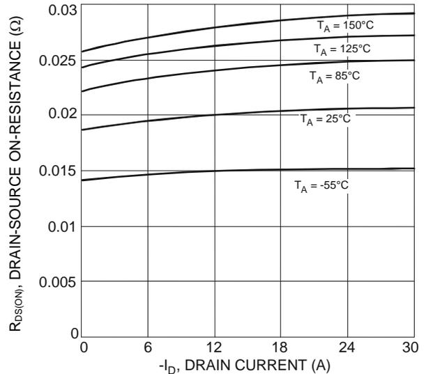
Fig. 4 Typical On-Resistance vs. Drain Current and Temperature
