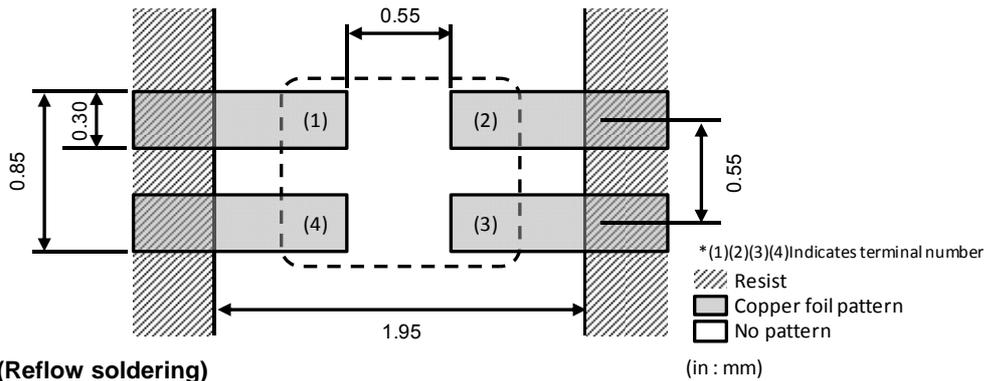
16.8 Soldering(Reflow soldering)
