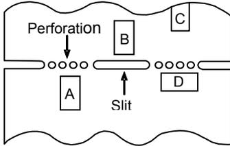
\*1 A > D is valid when stress is added vertically to the perforation as with Hand Separation.
