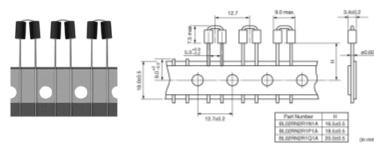
BL01/02/03 series are ferrite beads with lead wires to produce a high frequency loss for suppression of noise. Simple construction and easy-to-use, effective for low impedance circuits such as power supplies and grounds. Effective also for preventing overshoot and undershoot of digital signal in clocks or the like, and suppressing the higher harmonic wave. Suitable for prevention of abnormal oscillation at high frequency amplifying circuit.
