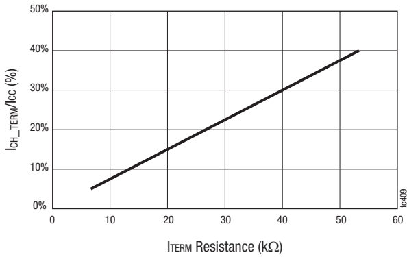
Figure 21. Termination Current to Constant Current Ratio (%) vs Termination Resistance
