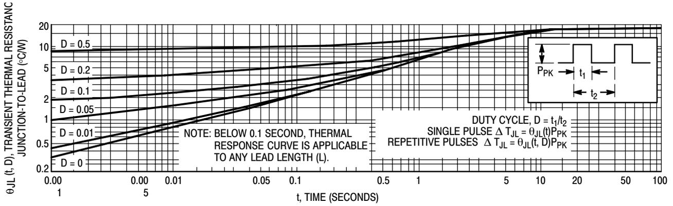
**Figure 4. Typical Thermal Response**
